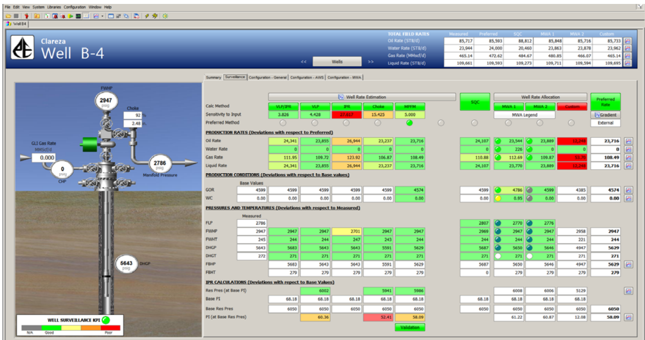
Fig 4. IVM well screen displaying a visualization of the well bore, real time data, multiple rate methods being calculated from the workflows along with the various validity checks for the different methods.
