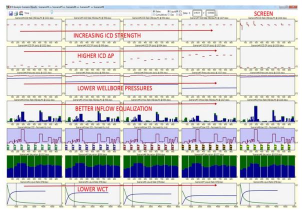
The cumulative oil production and final NPV go through a maximum with increasing ICD strength and then reduce: this suggests that there is an optimum ICD size for maximising NPV. These results are reasonable, since with higher ICD strength higher WCT/ high permeability regions are choked, giving us more oil. If the ICD pressure drop is excessive, then eventually we lose production due to the high choking.
