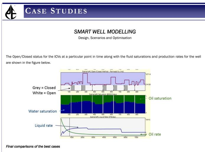
The figure below compares the NPVs for the ICV Open/Closed case (Scenario 1) with the ICV gradient method (Scenario 2) and the ICD genetic algorithm method (Scenario 3).
