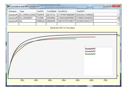
The ICV Open/Closed method yields the best NPV compared to all cases (including ICD, GA, ICV gradient cases) in this example. This will be expected, as continuously monitoring and controlling the well can give higher production than using a fixed device (ICD). The practicalities and economics of having the ability of dynamic control in the well will dictate the final design based on ICDs (GA - Scenario 3) or ICVs (Open/Closed - Scenario 1) for this case study.
