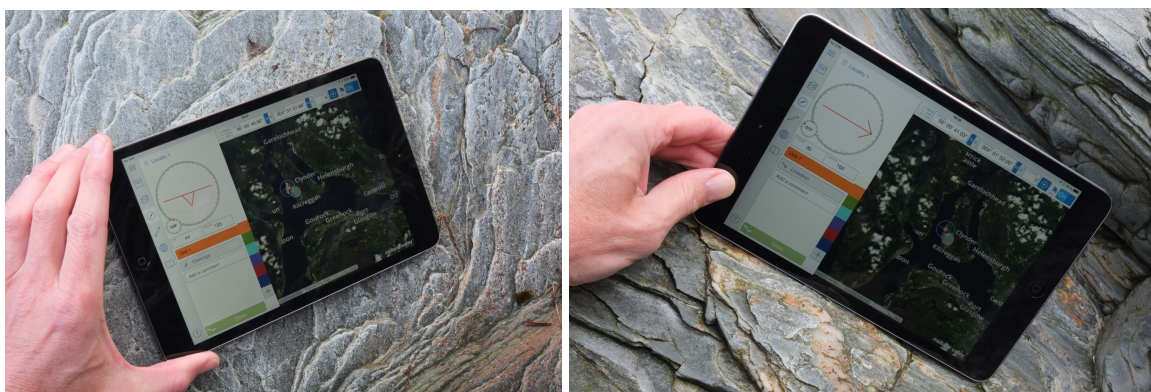
Figure: Photos showing the suitable tablet orientation when recording a planar (left) and linear measurement (right).
