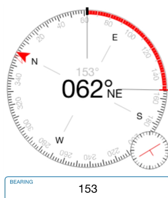
Figure: Compass face locked at a bearing of 153°. Once the compass has been locked, any deviation from the 153° bearing is shown by a red bar.
