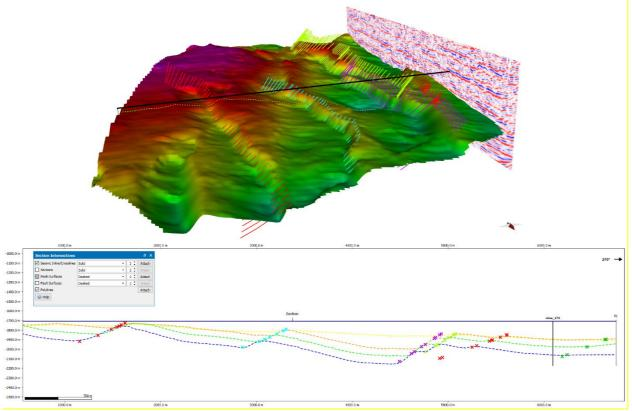
New Section Intersections tool. Allows for greater control of display of intersections in a Section View.
